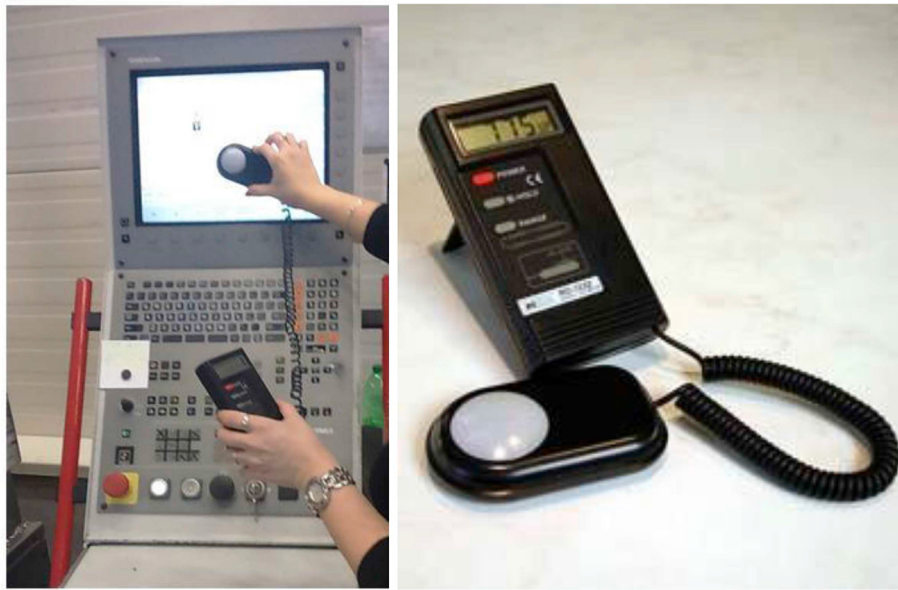
Fig. 2. Direct measurement of lighting (left) and Roline RO – 1332 - digital lux meter (right).
