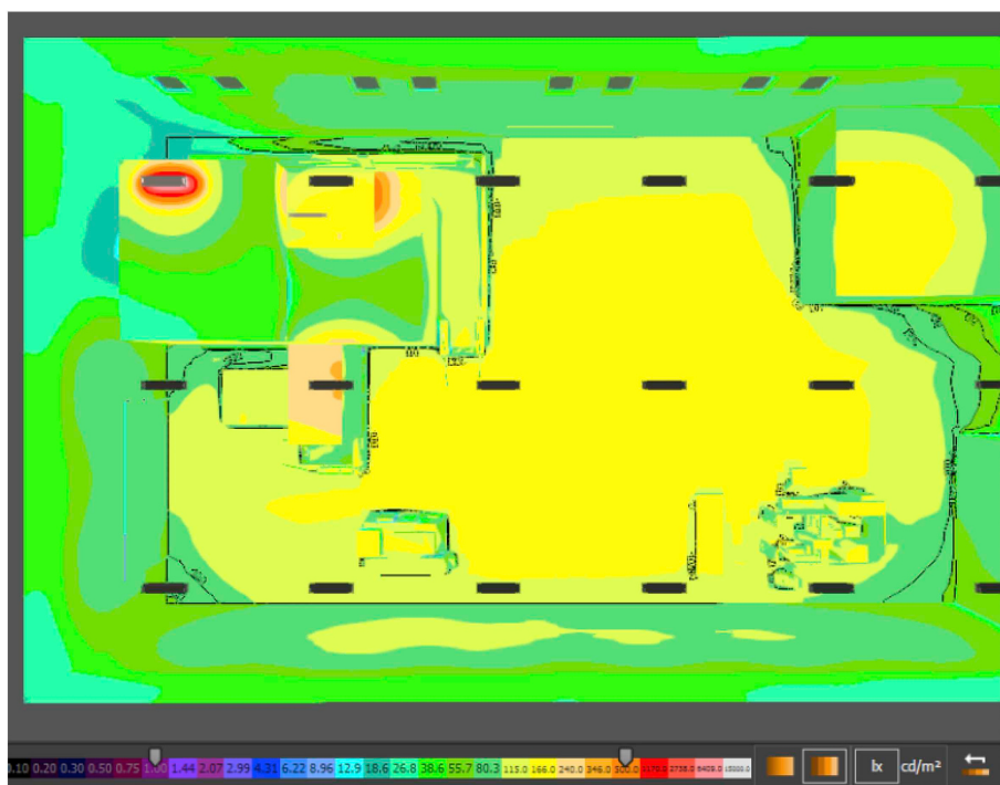
Fig. 8. 3D model of the isophote in the current state (artificial lighting).
