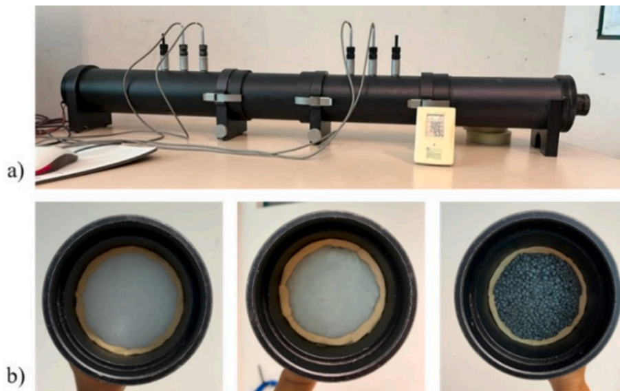
Fig. 4. a) Impedance tube, b) samples tested from left: PET, EF.PET, and I.EPS.
