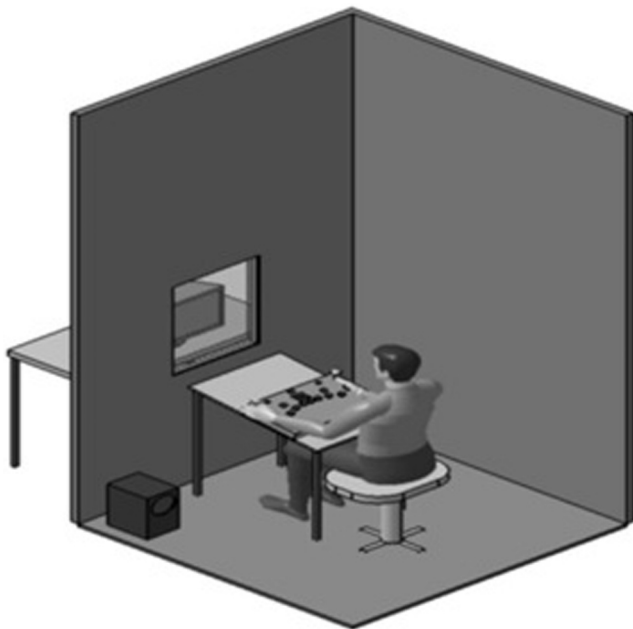
Fig. 1. Schematic figure of un-echoing room equipped with universal panel of VTS.
