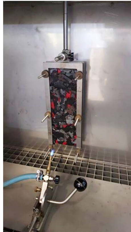
Fig. 5 Specimen placed in the frame for ignitability test
