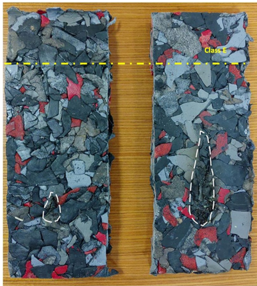
Fig. 10 Single-flame source (surface exposure) test results within 15 s (left) and 30 s (right) fire exposure. Burned areas are highlighted by white dotted lines
